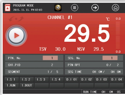
Fig. 37) Stop screen of program operation 2(Ch.1)
