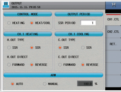
Fig. 85) Control output (Heating/cooling)
