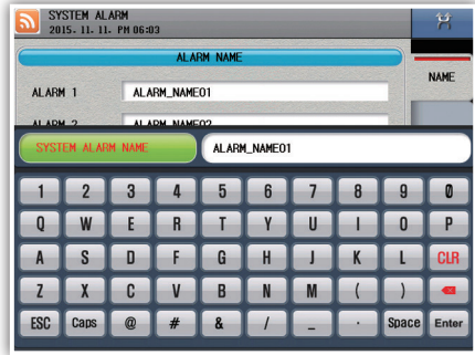
Fig. 112) Enter a system alarm name
